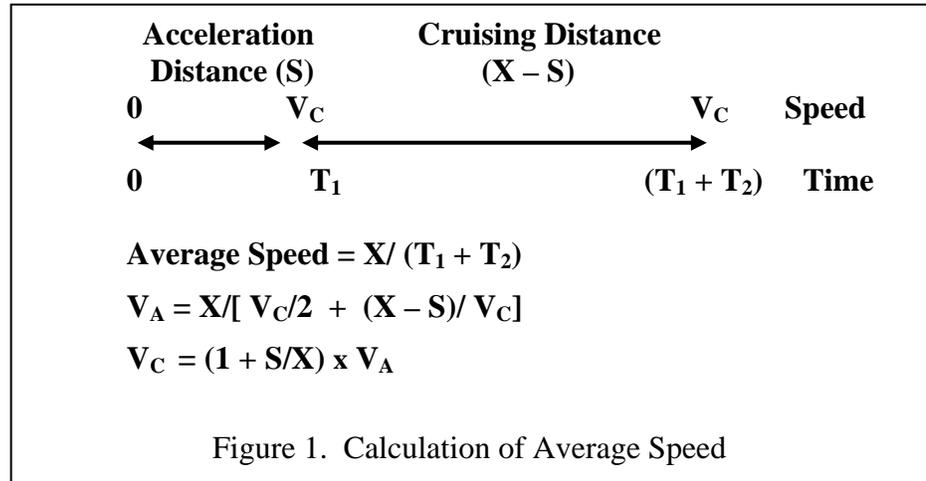
remainder of the distance, **X - S**, is the constant cruising speed **V<sub>C</sub>**. The corresponding times are the respective distances divided by their speeds, or
